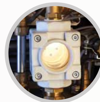
SIGHTGLASS TO CONTROL THE SOLVENT
